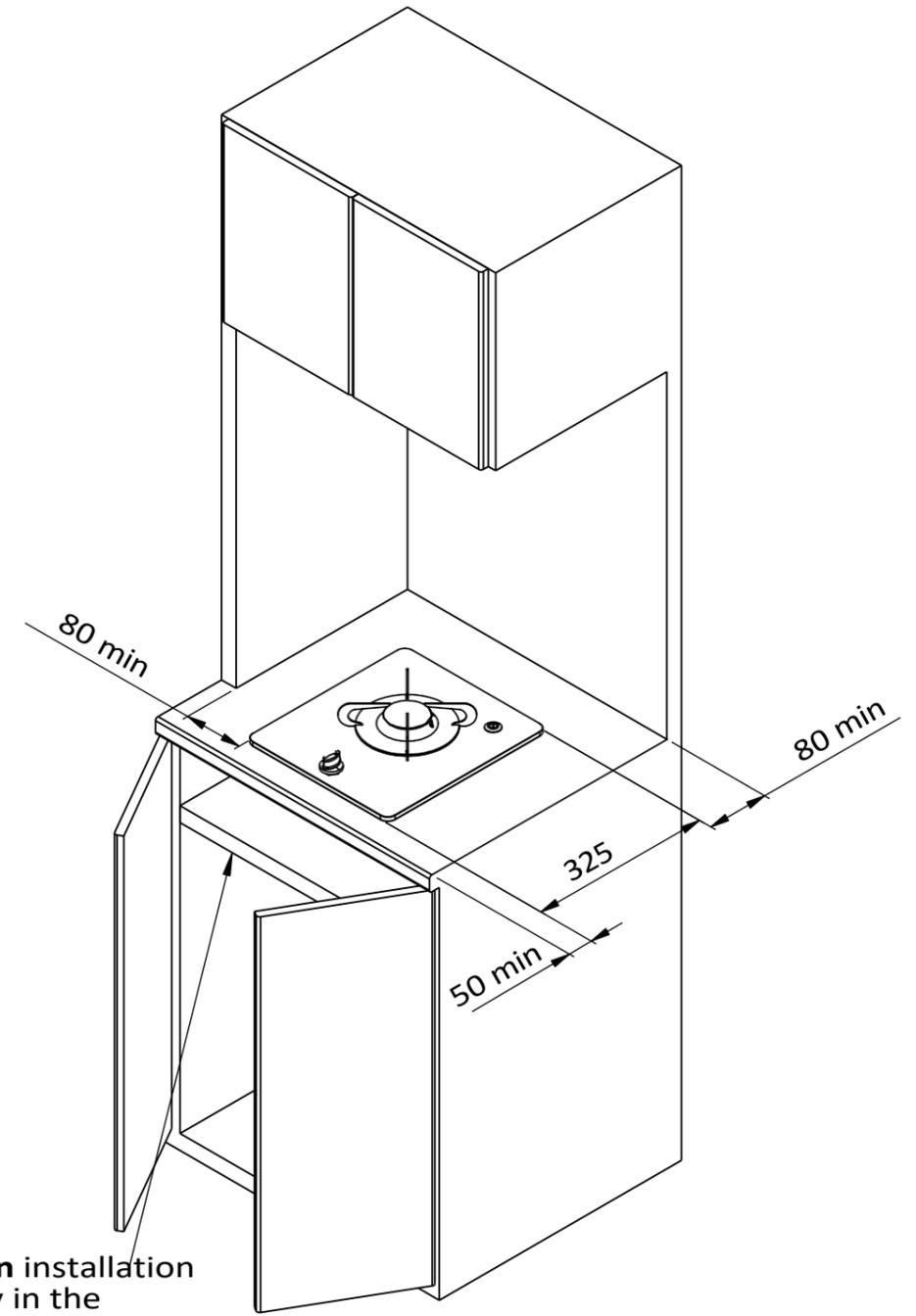
panel separation installation compulsory only in the presence of appliances below the hob
